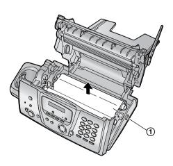
**6** Clean the thermal head (①) with a cloth moistened with isopropyl rubbing alcohol, and let it dry thoroughly.
